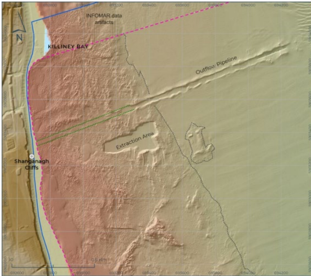
Figure 11 Shaded relief bathymetry offshore Shanganagh Cliffs (green dashed line shows outline of buried/covered pipeline. Grey dashed line shows outcrop extent (Source - Fugro and INFOMAR data)
